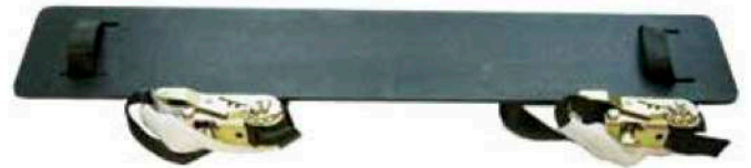
Boom Guard (24-03GUARD) Protects boom from saw damage. Mount on boom in front of tool holder to avoid damaging boom when inserting tool into holder. 32" X 5"
